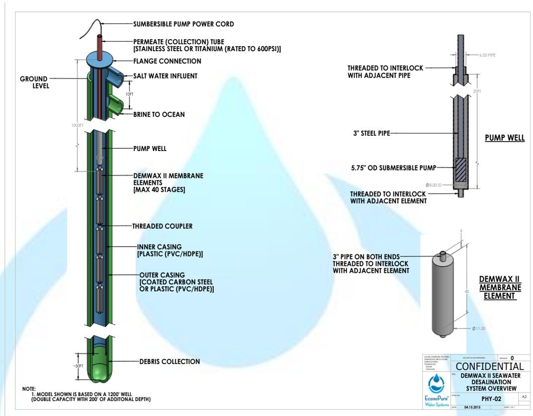
There should be several advantages to this development, the most important of which is the increase in square foot of membrane per available inner tube volume. It will directly increase output and efficiency.
