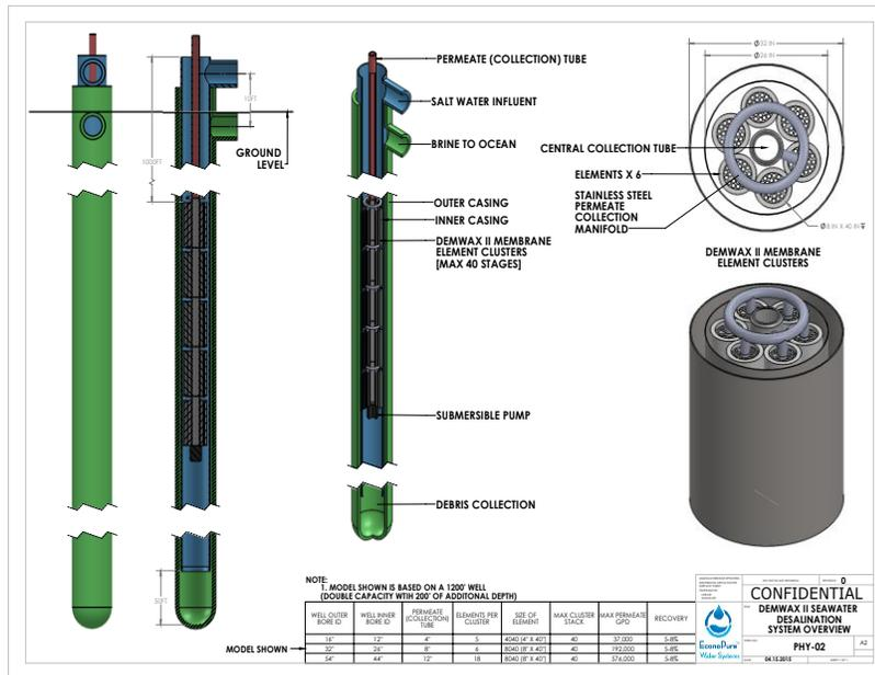
Figure 6 - DEMWAX II System Detail
