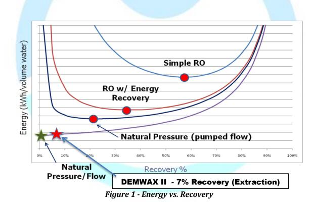
The final cost curve represents the case of the original DEMWAX<sup>M</sup> system, using natural static pressure in the sea, but also designed to capture natural movements of the feedwater. That system used the natural forces of gravity and currents in the ocean to naturally move the feedwater. In this case, the energy requirement tends toward the physical limit at a zero recovery.
